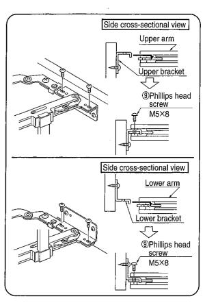
If the screws cannot be tightened downward when securing the upper door bracket, they can be tightened upward from under the joint. In that case, be sure to use the screw holes (inside the elliptical holes) in the upper door bracket.
