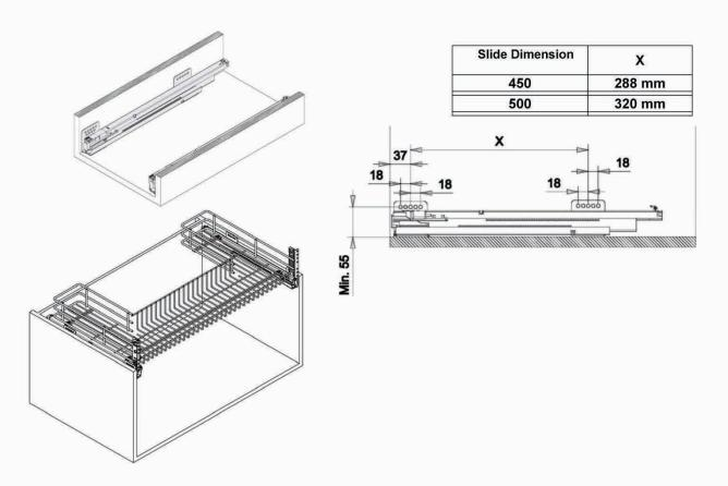
> Place covers over the slides. Place basket at the centre of the cabinet and screw it onto the covers
