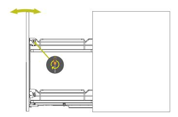
Loosen the 3.9x13 screws, to adjust the door to the right and left.
