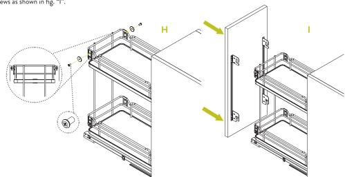
Loosen the four screws M6x10 "L", turn the screw "M" as shown to adjust the door up and down.
